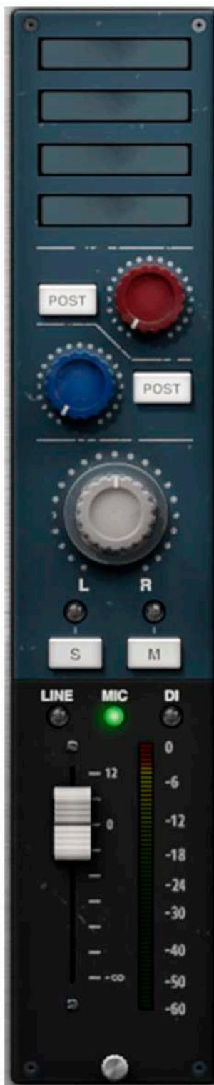
Starting on the left hand side you'll find the channels for each of the i73 Interface's inputs. Each of these inputs can be recorded into your DAW onto two tracks simultaneously, one processed and the other not. This provides the user with options previously unheard of while allowing one to quickly treat a signal for the session at hand, keeping things moving, but still maintaining a clean, unprocessed version of the same, that can be perfectly processed at a latter, more convenient time.
