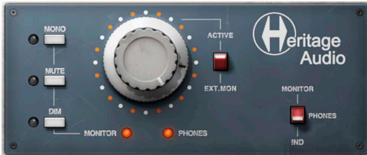
At the top on the right-hand side is where you have total control over the actual monitoring itself. Here you set the individual volumes for each output with the concentric knobs representing either MONITOR and PHONES.
