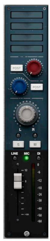
Starting on the left hand side you'll find the channels for each of the i73 Interface's inputs. Each of these inputs can be recorded into your DAW onto two tracks simultaneously, one processed and the other not. This provides the user with options previously unheard of while allowing one to quickly treat a signal for the session at hand, keeping things moving, but still maintaining a clean, unprocessed version of the same, that can be perfectly processed at a latter, more convenient time.
