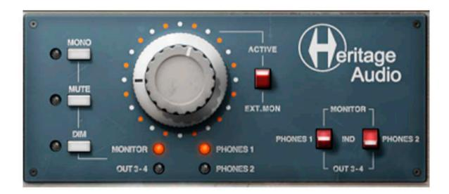
At the top on the right-hand side is where you have total control over the actual monitoring itself. Here you set the individual volumes for each output with the concentric knobs representing either MONITOR and PHONES 1 or OUT 3&4 and PHONES 2.
